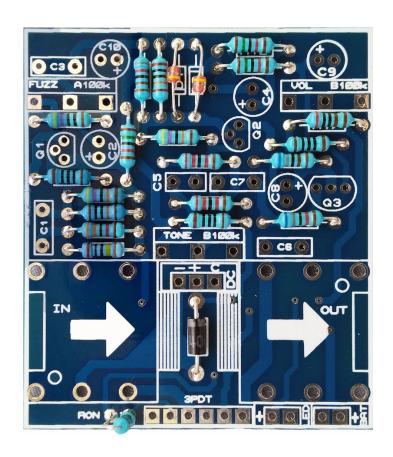
Place the resistors and diodes. If you have troubles reading the values, check out our "Reading Part Values" tutorial.
