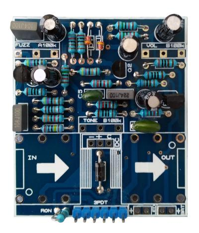
Solder the capacitors and transistors. If you have troubles reading the values, check out our <u>"Reading Part Values"</u> tutorial. Pay attention to the orientation, as well as to the polarity for electrolytic capacitors.
